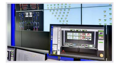
JST MultiConsoling<sup>®</sup>: The photo shows the JST myGUI, the user interface for the MultiConsoling<sup>®</sup> computer is simply and intuitively connected to the workplace monitors and the large-screen displays. Only one mouse and keyboard is required per workstation.
