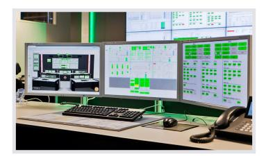
JST MultiConsoling®: The myGUI – shown here on the left screen – serves as a user interface for MultiConsoling®, with which it is possible to display any sources (computers, cameras, etc.) in real time on the workplace monitors, on individual large-screen displays or as BigPicture across several large-screen displays. Another special feature: Only one mouse and keyboard are needed for each workstation to operate everything in real time.
