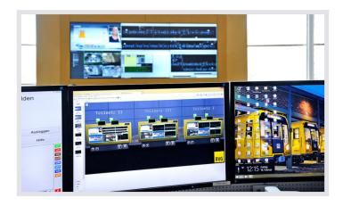
JST <u>MultiConsoling</u>®:myGUI – shown here on the middle screen – serves as the user interface for <u>MultiConsoling</u>®, with which it is possible to display any sources (computers, cameras etc.) in real time on the workstation monitors, on individual <u>large-screen displays</u> or as BigPicture across several large-screen displays.
