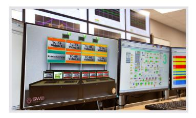
ST MultiConsoling®: The myGUI – shown here on the left screen – serves as the user interface for the JST MultiConsoling®. Advantage of this technology: Computer signals with keyboard, video, mouse, audio signals, cameras and even TVs are flexibly displayed in real time on the monitors at the workplace or on the large display walls.
