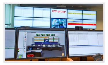
**JST**<u>control center desk</u>: A special solution in the Otto Group control center desk – the workplace displays are located on a height-adjustable monitor surface that can be raised and lowered as required.
