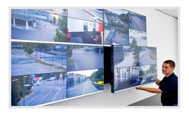
JST QuickOut mounting system: The <u>large sreen displays</u> are mounted directly on the wall in a way that saves space. By applying light pressure to the outer edges of the display, each individual display slides forward (Quick-Out) to provide access to rear connections and technical components in case of revision.
