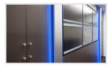
JST large display wall covering: In the integrated control center of Stadtwerke Gießen, the cladding of the <u>large display screen</u> not only reduces the noise level in the control room, but also offers <u>additional storage space</u> thanks to its multifunctional design with hinged doors.
