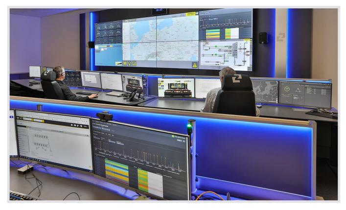
JST control room solution: real-time monitoring, data analyses, precise availability forecasts - with the support of the Jungmann team, <u>state-of-the-art solutions</u> were implemented in Zeppelin Power Systems' new <u>Fleet Operations Center</u> for the <u>service of globally monitored drive and power systems</u>. Goal: To support Predictive Maintenance.
